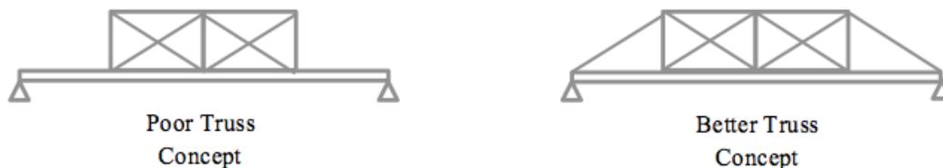
Figure 4.2: Think about where the load is applied, and how it will be transferred through your structure.
